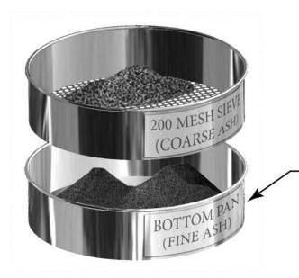
PLACE 10 GRAMS OF ASH ON STACKED 200 MESH PAN AND SHAKE FOR 20 MINUTES
